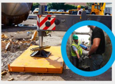
We've recently taken delivery of PANDA®, a particularly useful and flexible dynamic cone penetrometer (DCP) device which will supplement the TRL probe that has been part of our insitu test kit for over 10 years.
